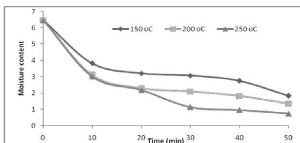
**Fig. 1:** Changes in the moisture content of cocoa beans during superheated steam roasting at different temperatures (150, 200 and 250 °C) for 50 min.
