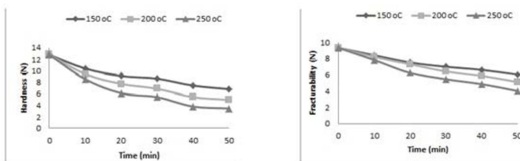
**Fig. 3:** Effect of temperature and time on the hardness and fracturability of cocoa beans during superheated steam roasting at different temperatures (150, 200 and 250 °C) for 50 min.
