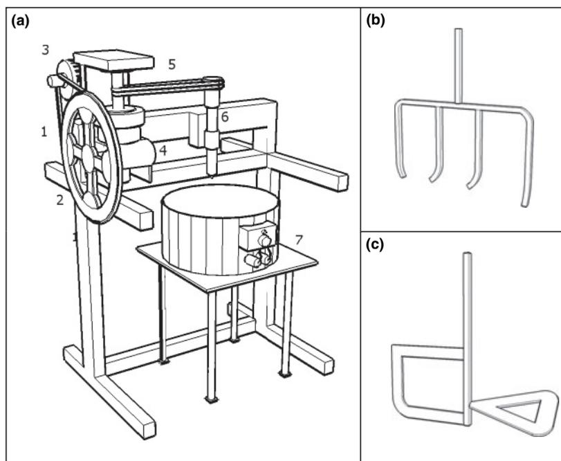
**Figure 1** The laboratory scale conch project. (a) General scheme of the equipment showing seven principal parts: (1) leather strap A57, (2) pulley, (3) induction motor, (4) speed dropbox, (5) leather straps ZX785, (6) axle with mandrill and (7) thermostatic bath; (b) yoke-type impeller; (c) propeller-type impeller.
