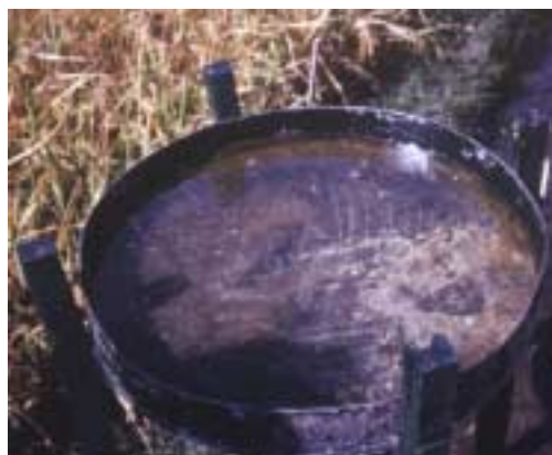
Figure 6.12 Champion Water Trap , without lid. Solid construction, high capacity, ideal for research purposes but in common with all water traps requires high level of maintenance and insect identification can be problematic if oil is added to water. Alternatives include surfactants such as washing detergents. (NRI, University of Greenwich, UK)
