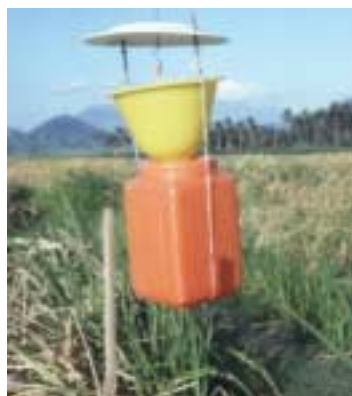
Figure 6.1 Funnel trap. Made in plastic from inverted white plate (lid) yellow funnel, and opaque orange container for retaining insects. The funnel is held in place on the lid of the plastic container by a ring clip or rubber band. Widely used by NRI in Pakistan, Africa and south east Asia in 1980s and 90s, produced from locally available materials.
