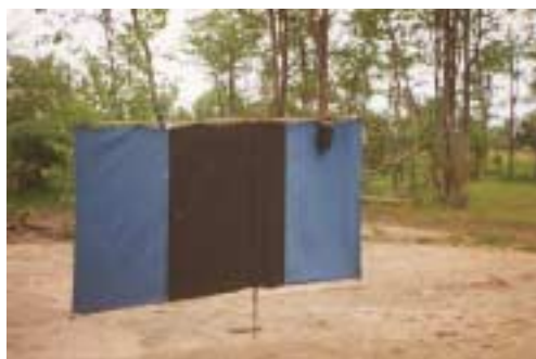
Figure 6.25 Insecticide-impregnated target for tsetse fly. Primarily used for control because insects landing on the target surface are killed by exposure to the insecticide but not retained in the vicinity of the target. The blue colour is highly attractive to the diurnal flying insects, while they preferred to land on black. The target is pivoted because tsetse are attracted by moving objects and coated with insecticide as a killing agent. The pyrethroid used for killing the insects is suitably formulated to withstand photo-degradation and rain. (NRI, University of Greenwich, UK)
