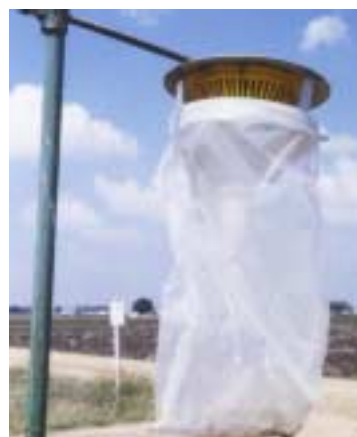
Figure 6.4 Double funnel trap. Made from inverted metal plate (lid), yellow funnel with slits to allow pheromone out from a lure. The yellow and white funnels act to direct the insects into the retaining plastic bag. Early versions of the trap design used widely in Egypt had problems with the plastic bags that split under intense sunlight and wind action. ICRISAT Design ( Heliothis trap).
