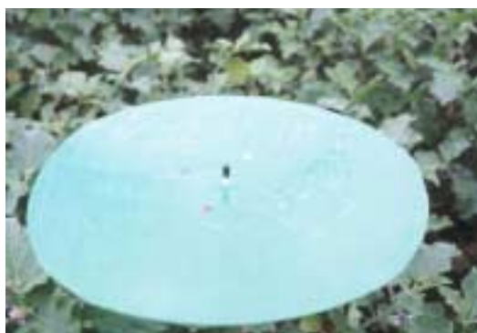
Figure 6.9 Sticky disc trap. Highly efficient but saturating design limits trap catch and open surface susceptible to build-up of debris. Lure protection relied on black paint applied to base of pheromone lure. (NRI, University of Greenwich, UK)
