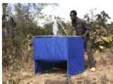
Figure 6.26 Tsetse fly entry trap for assessing population densities and species composition of insects attracted by the olfactory and visual cues presented by the trap. Flies entering the trap are attracted by light from above and move upward and are retained in the transparent collecting vessel. (NRI, University of Greenwich, UK)
