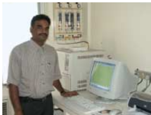
Figure 4.2 Quantitative GC analysis of compounds ensures high quality products. Note filters to purify carrier gases. Courtesy of SunAgro Pvt Ltd.
