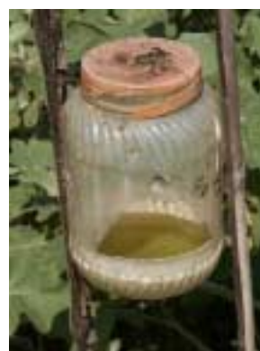
Figure 6.14 Alam water trap . Care should be taken over the choice of container because some locally produced plastics are not stable under intense sunlight, the loss of plasticiser can cause the fabric of the traps to become brittle, as seen in this prototype. (Trap courtesy Dr N. S. Alam, BARI, Bangladesh)
