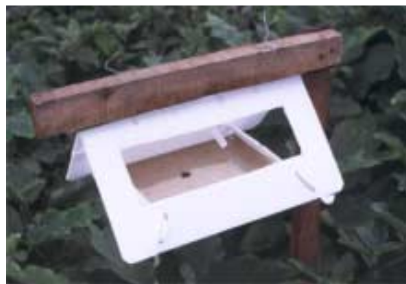
Figure 6.6 Open-delta trap. This modified Delta trap was found to catch Brinjal borer, L. orbonalis and rice stem borer, S. incertulas more efficiently than the conventional Delta trap but in common with the conventional Delta trap has a limited capacity that reduces its usefulness for field applications. Adhesives such as 'Tangle Foot' are unaffected by sunlight and are rain-fast. The adhesive is not available in South Asia although is widely available, at low cost, on the international market. (NRI, University of Greenwich, UK)
