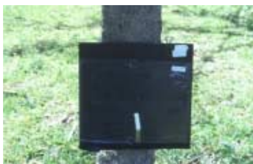
Figure 6.27 Odour-baited sticky target. Black sticky plates used for catching New World Screwworm (NWSW) in Mexico. Experimental lures were applied to simple cotton wicks. A 0.5 x 0.5 m square could catch up to 1000 insects. (NRI, University of Greenwich, UK)
