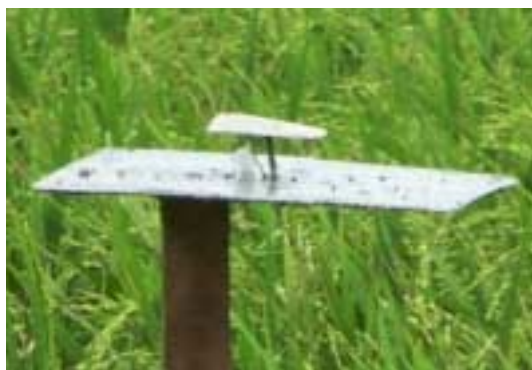
Figure 6.7 Sticky plate trap. Prototype trap developed by Syngenta Bangladesh Limited for use with yellow rice stem borer. Cost-effective trap design produced from local materials. Required only single support and lures were well protected. (Trap courtesy of Syngenta Bangladesh Limited)
